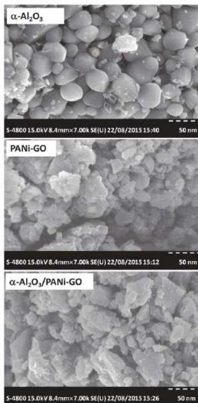
Fig. 2. FE-SEM images of \alpha\text{-Al}_2\text{O}_3 , PANI-GO and \alpha\text{-Al}_2\text{O}_3 /PANI-GO composite.
